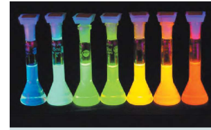
? These containers hold solutions of microscopic semiconductor particles of different sizes. The particles glow when exposed to ultraviolet light; the smallest particles glow blue and the largest particles glow red. Why?
